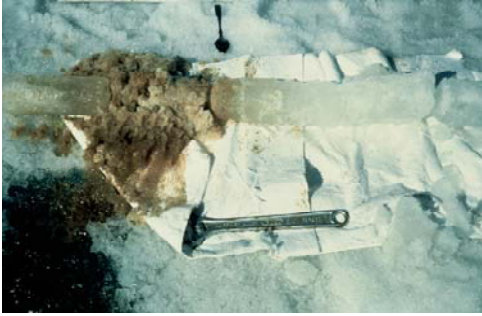
Core Showing New Ice Growth Encapsulating Canadian Experiment Oil in Ice
