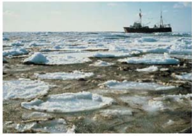
Oil in slush among pancake ice off the Canadian East Coast, 1986 (SL Ross and DF Dickins, 1987)
