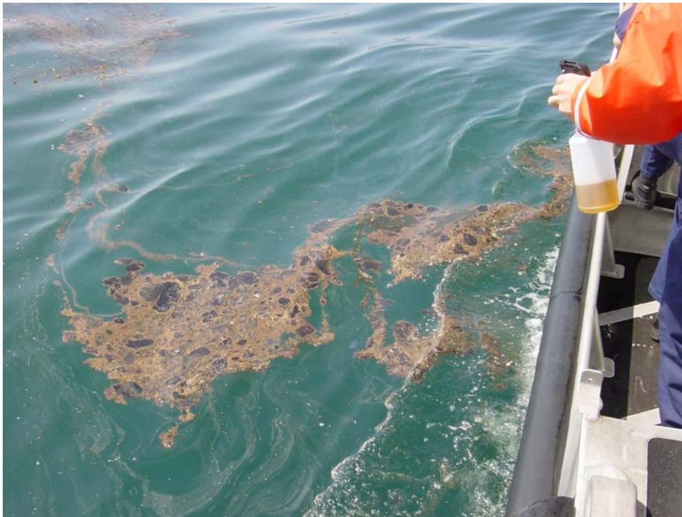
Figure 37. Testing on heavier, naturally accumulated patches of oil. Some patches were created by earlier winds and resulting convergence zones; other from the splashing effects of water off the sides of the boat.
