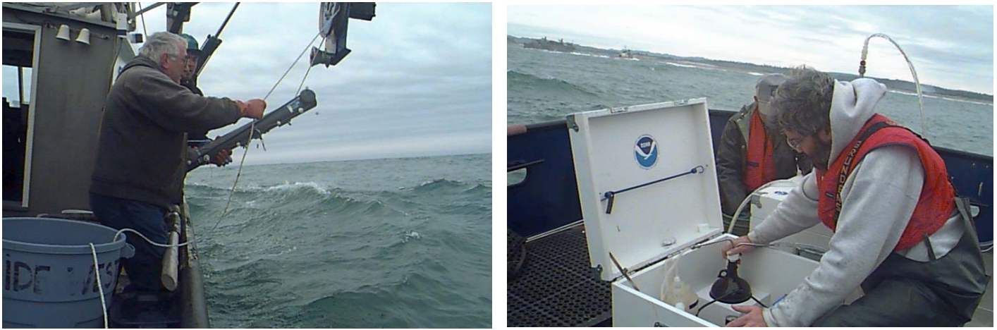
Figure 3. Use of a conventional 4-Liter Go Flo ® Bottle connected to the PLVWSS to obtain discrete samples of dispersed oil droplets and dissolved components at different water depths following the 1999 M/V New Carissa oil spill off Coos Bay, OR.
