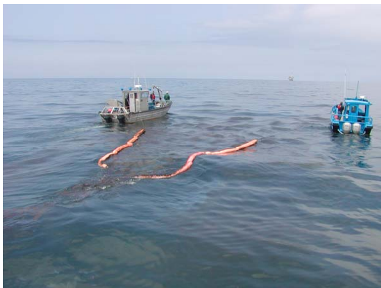
Figure 31. Attempt to simulate the NeatSweep boom arrangement to determine if the oil would stick irreversibly to the boom or flow through the opening at the apex.
