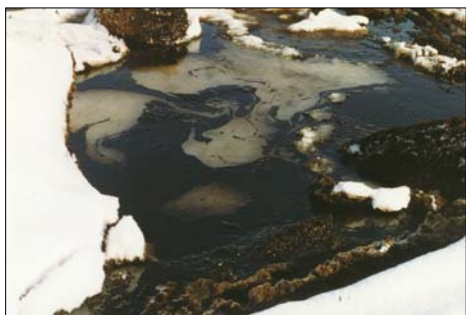
Figure 2. Observed distribution of oil and water above ice at 24 hours Source: M. Reed, SINTEF, 1993
