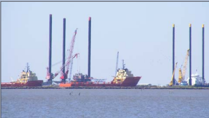
Jack-up barges used to bring supplies to offshore oil platforms, Port Fourchon, LA.
